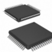
MC68HC908LV8CPBE NXP USA Inc. IC MCU 8BIT 8KB FLASH 52LQFP
