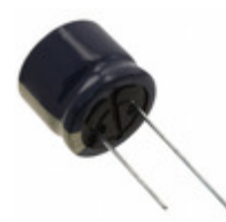
EEU-FC1C392SB Panasonic Electronic Components CAP ALUM 3900UF 20% 16V RADIAL
