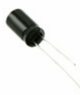
25PX220MEFCTA6.3X11 Rubycon CAP ALUM 220UF 20% 25V RADIAL
