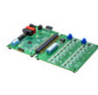
ADM1266-EVALZ ADI (Analog Devices, Inc.) EVALUATION BOARD
