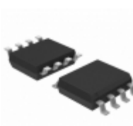
MCP6V01T-E/SNVAO Micrel / Microchip Technology IC OPAMP CHOPPER 1.3MHZ 8SOIC
