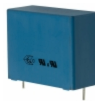
B32916A4564M EPCOS (TDK) CAP FILM 0.56UF 20% 440VAC RAD
