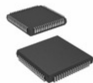
CY7C4245-15JXC Cypress Semiconductor Corp IC SYNC FIFO MEM 4KX18 68-PLCC
