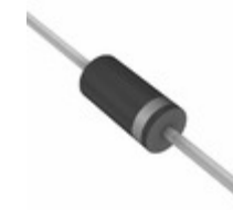
FR153G A0G TSC (Taiwan Semiconductor) DIODE GEN PURP 200V 1.5A DO204AC
