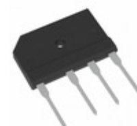
TS8P05GHD2G TSC (Taiwan Semiconductor) BRIDGE RECT 1PHASE 600V 8A TS-6P
