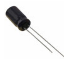
EEU-FC1C121H Panasonic Electronic Components CAP ALUM 120UF 20% 16V RADIAL
