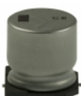
EEV-EB2E220SM Panasonic Electronic Components CAP ALUM 22UF 20% 250V SMD
