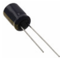
EEU-FC1H680BJ Panasonic Electronic Components CAP ALUM 68UF 20% 50V RADIAL
