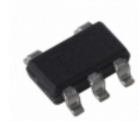
MIC5252-1.8YM5-TR Microchip Technology IC REG LDO 1.8V 0.15A SOT23-5
