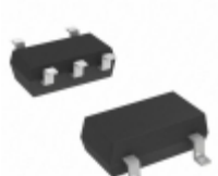
AN80L51RMS Panasonic Electronic Components IC REG LDO 5.1V 0.15A MINI5D
