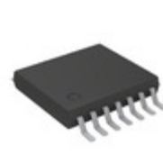
MCP4661-502E/ST Microchip Technology IC DGTL POT 5K 257TAPS 14-TSSOP
