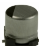
EEV-HA1E330WR Panasonic Electronic Components CAP ALUM 33UF 20% 25V SMD
