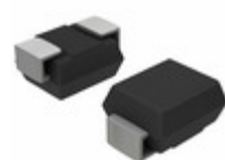
CD214B-T40ALF Bourns Inc. TVS DIODE 40VWM 64.5VC DO214AA
