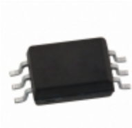
ACPL-W611-000E Avago Technologies (Broadcom Limited) OPTOISO 5KV OPEN COLLECTOR 6SO
