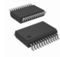
AD7225CRS Analog Devices Inc. IC DAC 8BIT QUAD W/AMP 24-SSOP
