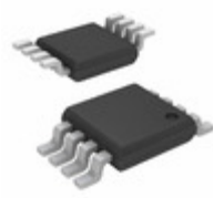
MIC5208-3.8YMM Microchip Technology IC REG LDO 3.8V 50MA 8MSOP
