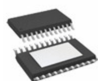
AD5724RBREZ-REEL7 Analog Devices Inc. IC DAC 12BIT DSP/SRL 24TSSOP
