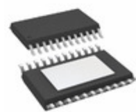
AD5724AREZ-REEL7 Analog Devices Inc. IC DAC 12BIT DSP/SRL 24TSSOP
