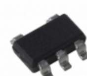
MIC5245-2.6YM5-TR Microchip Technology IC REG LDO 2.6V 0.15A SOT23-5
