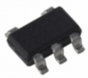
MIC5245-2.7YM5-TR Microchip Technology IC REG LDO 2.7V 0.15A SOT23-5
