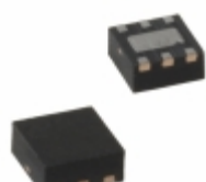
MIC5318-1.5YMT-TR Microchip Technology IC REG LDO 1.5V 0.3A 6TMLF
