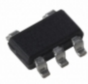
MIC5317-3.3YM5-TR Microchip Technology IC REG LDO 3.3V 0.15MA 5SOT23
