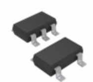
MIC5318-1.5YD5-TR Microchip Technology IC REG LDO 1.5V 0.3A TSOT23-5
