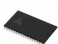
AS7C4098A-20TCN Alliance Memory, Inc. IC SRAM 4MBIT 20NS 44TSOP
