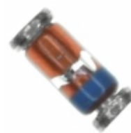
DL5236B-TP Micro Commercial Co DIODE ZENER 7.5V 500MW MINIMELF
