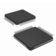
AT87C51RD2-RDTUL Microchip Technology IC MCU 8BIT 64KB OTP 64LQFP
