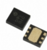
XC6121D746ER-G Torex Semiconductor Ltd IC WATCHDOG TIMER 6-USP
