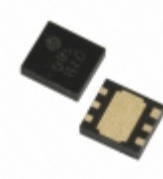
XC6121D748ER-G Torex Semiconductor Ltd IC WATCHDOG TIMER 6-USP
