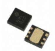
XC6121D743ER-G Torex Semiconductor Ltd IC WATCHDOG TIMER 6-USP
