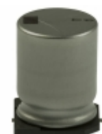
EEV-EB2E470M Panasonic Electronic Components CAP ALUM 47UF 20% 250V SMD
