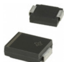
SM15T220A-M3/57T Vishay Semiconductor Diodes Division TVS DIODE 188VWMM 328VC DO214AB
