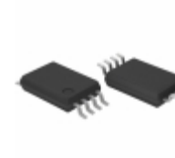
BR25L020FV-WE2 Rohm Semiconductor IC EEPROM 2KBIT 5MHZ 8SSOPB
