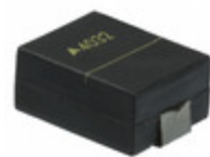
CU4032K140G2K1 EPCOS (TDK) VARISTOR 220V 1.2KA 4032
