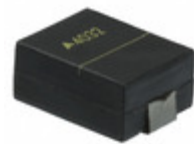
CU4032K175G2 EPCOS (TDK) VARISTOR 270V 1.2KA 4032
