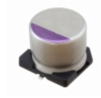
63SXV39M Panasonic SXV SERIES - OSCON SMD TYPE 63V
