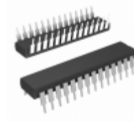
PIC16C55-10I/SP Microchip Technology IC MCU 8BIT 768B OTP 28SDIP
