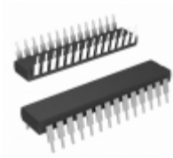
PIC16C55-10E/SP Microchip Technology IC MCU 8BIT 768B OTP 28SDIP
