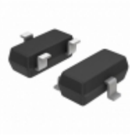
MMBZ5230BLT3G ON Semiconductor DIODE ZENER 4.7V 225MW SOT23-3
