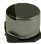
ECE-V1HA220UP Panasonic Electronic Components CAP ALUM 22UF 20% 50V SMD
