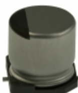
EEE-1VA101P Panasonic Electronic Components CAP ALUM 100UF 20% 35V SMD
