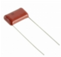
ECQ-E6563JFB Panasonic Electronic Components CAP FILM 0.056UF 5% 630VDC RAD
