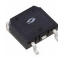
APT42F50S Microsemi Corporation MOSFET N-CH 500V 42A D3PAK
