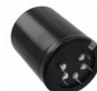
ECE-P2WA102HA Panasonic Electronic Components CAP ALUM 1000UF 20% 450V SNAP
