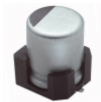
MZA50VC4R7MD61TP United Chemi-Con CAP ALUM 4.7UF 20% 50V SMD
