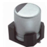
MZA6.3VC471MH10TP United Chemi-Con CAP ALUM 470UF 20% 6.3V SMD
