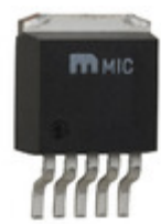
MIC5209-3.0YU Microchip Technology IC REG LDO 3V 0.5A TO263-5
