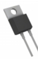
SCS215KGC Rohm Semiconductor DIODE SCHOTTKY 1.2kV 15A TO220AC
