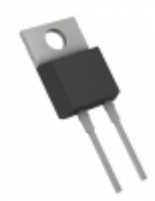
SCS212AGHRC Rohm Semiconductor DIODE SCHOTTKY 650V 12A TO-220-2
