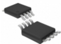
LTC6652BHMS8-2.5#PBF Linear Technology IC VREF SERIES 2.5V 8MSOP
