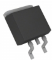
BA17810FP-E2 LAPIS Semiconductor IC REG LDO 10V 1A TO252-3
