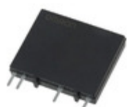
G3MC-201PL-VD DC24 Omron Automation and Safety RELAY MINI SSR 1A 24VDC PCB
