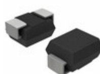
SMBJ85A Bourns Inc. TVS DIODE 85VWM 137VC DO214AA
