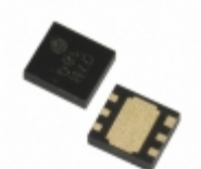
XC6121C449ER-G Torex Semiconductor Ltd IC WATCHDOG TIMER 6-USP
