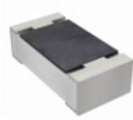
RT0603BRD07221KL Yageo RES SMD 221K OHM 0.1% 1/10W 0603
