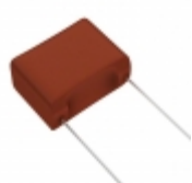
ECW-F2W275JA Panasonic Electronic Components CAP FILM 2.7UF 5% 450VDC RADIAL
