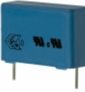
B32923A2334M EPCOS (TDK) CAP FILM 0.33UF 20% 305VAC RAD
